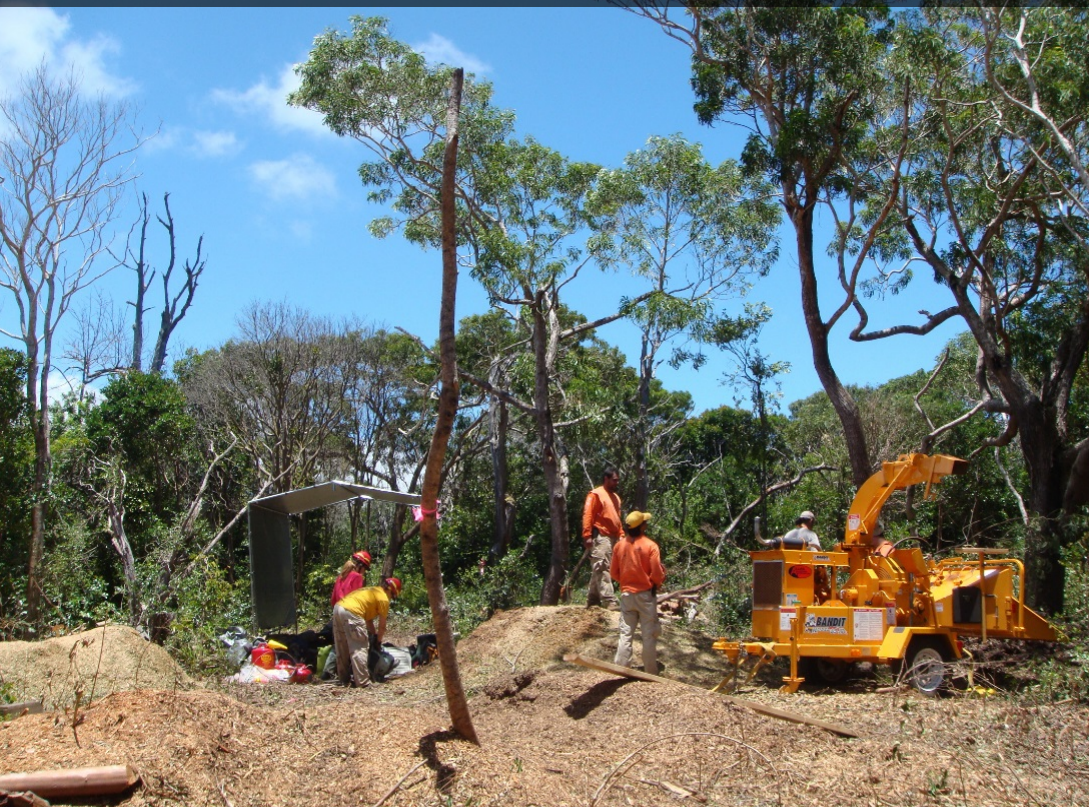
The chopper easily handled 6" diameter trunks.
